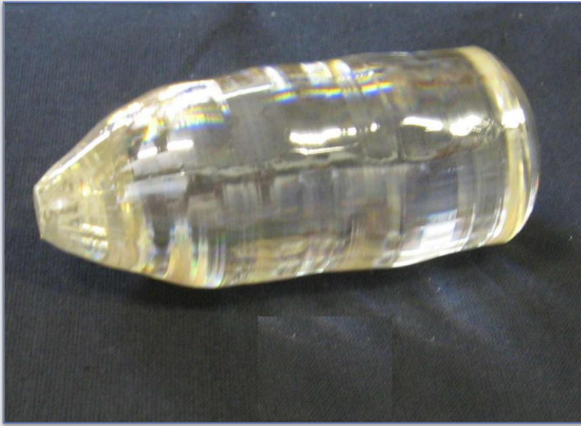
Large volume ZnWO 4 crystal scintillators up to \varnothing 50 \times 100 mm
