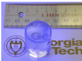
Fig. 1. Cerium-activated gadolinium bromide glass-matrix cylinder, 2.5-cm dia. × 3.0-cm height, under 365 nm UV illumination.
