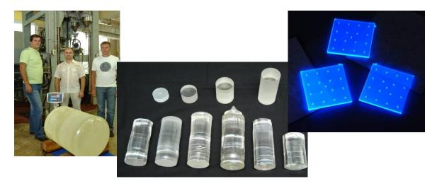
Unique technologies and equipment for automated growth and tooling of large single crystals of high structural perfection, which allow us to obtain alkali halide scintillation crystals with a diameter exceeding 500 mm and weight over 500 kg, have been introduced.
