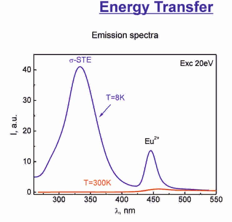
Excitation efficiency decreases with the temperature growth (see left fig.). It looks like STE luminescence quenching. Exciton transfer is not visible at all at RT. At the same time the contribution of electron-hole mechanism both at low and at room temperature is insignificant.
