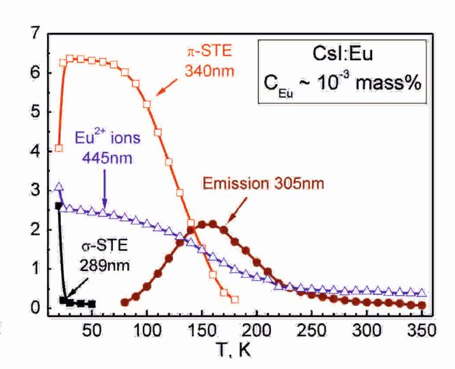
Spectra of isovalent (Na<sup>+</sup>, Tl<sup>+</sup>, In<sup>+</sup>) [4] and divalent (Eu<sup>2+</sup>) doped crystals are significantly different.
